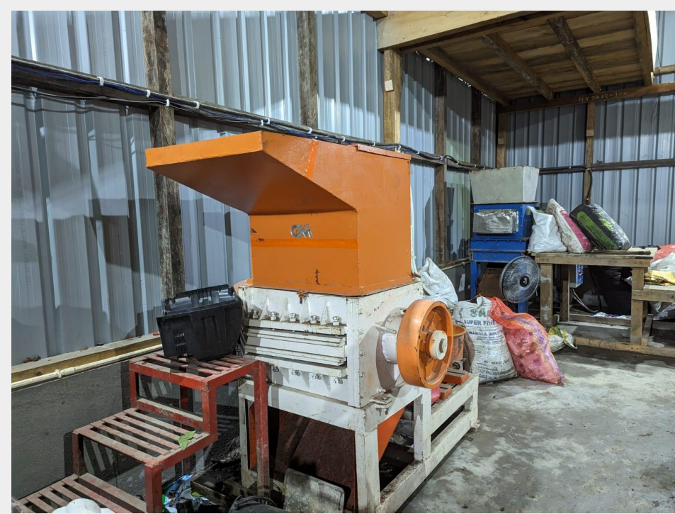
Reject waste will be shredded and/or ground.
